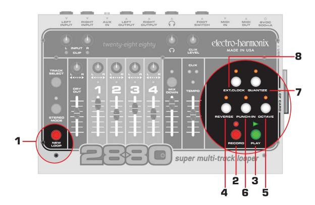
1. NEW LOOP Button: The NEW LOOP button will put the 2880 into Record-Ready Mode. When you press the NEW LOOP button, the RECORD LED will blink rapidly, telling you the 2880 is ready to record. Press the NEW LOOP button again to exit Record-Ready Mode. If you press the NEW LOOP button while recording a New Loop it will end recording and put the 2880 into Playback mode. Below is a table displaying the results of pressing the NEW LOOP button depending on the current mode of the 2880:
